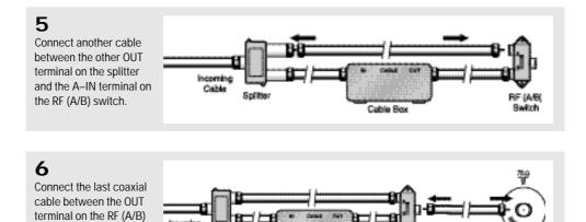
Switch and the VHF/UHF terminal on the rear of the TV.
